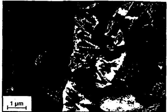
Fig. 11—Centered dark field TEM micrograph of weld metal 0.12%C—2.2%Mn, showing an almost continuous layer of retained austenite.
