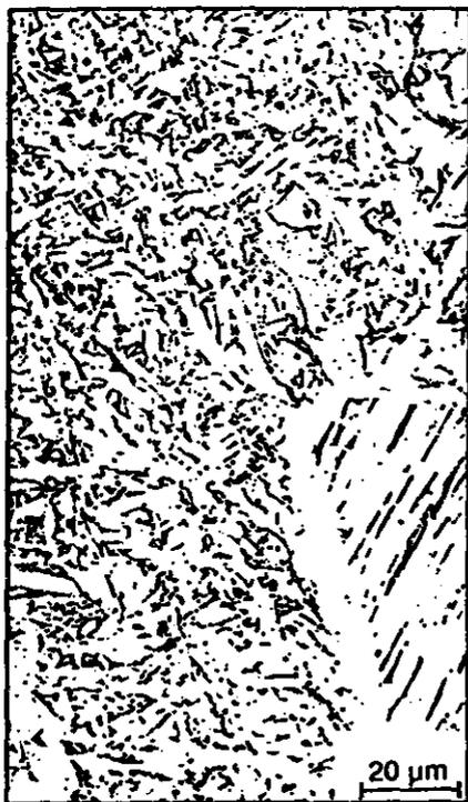
Fig. 5—Optical micrograph of the weld metal with 0.03% C—0.8% Mn. The microstructure consists mainly of a coarse allotriomorphic ferrite, ferrite side plates and coarse acicular ferrite.
